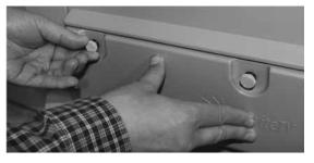
Press firmly on the cover, and secure the Thumb Screws tightly.
